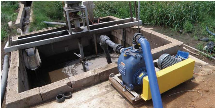
*The Gorman-Rupp T2A3-B pump was fitted with a 4kW motor to provide the flow and pressure needed.*
