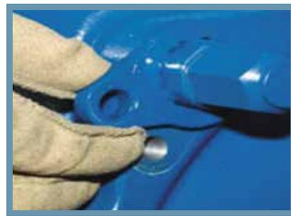
***Just remove the locking screw, rotate the collar by two notches and replace the screw. One operator with two spanners takes five minutes and the pump is back to peak efficiency. The pump is NOT removed from the piping system.***
