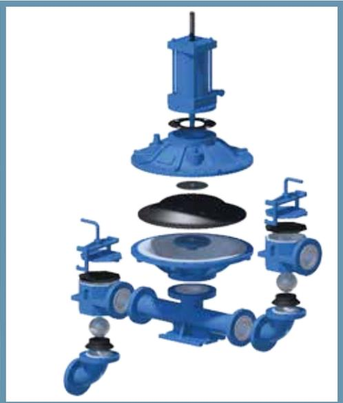
Pumps are available with wetted surfaces lined or unlined. Pumps can be lined in Hypalon, Nordel, Neoprene, Nitrile or Viton for better abrasion resistance and mild corrosive service. For the best chemical and abrasive resistance in acid or organic slurries, pumps can be lined in ETFE fluoropolymer (aka - Tefzel®).
