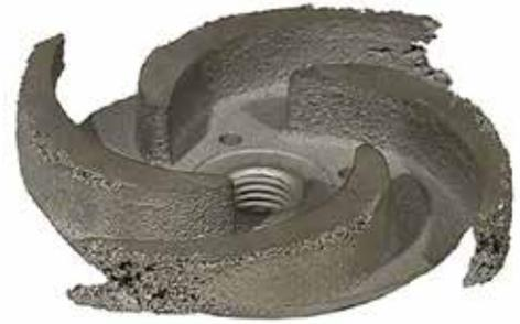
An impeller showing signs of “tip” cavitation.
