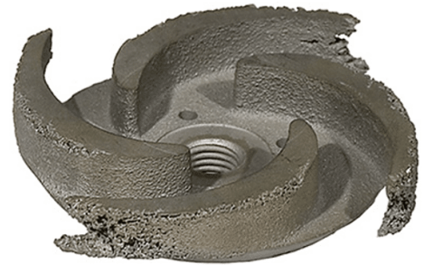
An impeller showing signs of “tip” cavitation.
