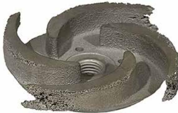
An impeller showing signs of “tip” cavitation.
